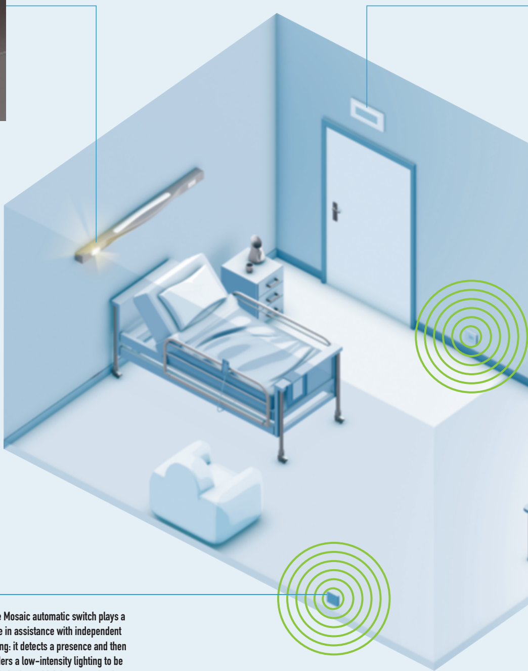
Signalling bulkhead light with low-intensity lighting integrated into the bedhead strip.
