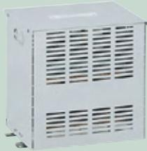
**When the sum of the leakage currents of the devices supplied via the part of an installation protected by an RCD is likely to be greater than half the rated residual current ( $I_{\Delta n}$ ) for this RCD, there is a high risk of tripping. This problem can be avoided by using a circuit separation transformer, under TN-S neutral earthing system conditions.**
