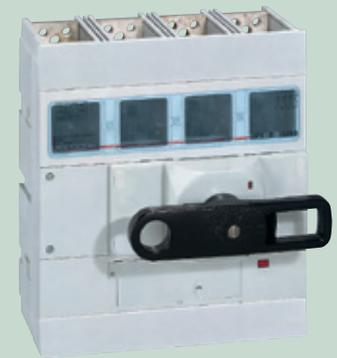
Isolating switches in the Vistop range (up to 160 A) and the DPX-I range (up to 1600 A) are particularly suitable for switching circuits that have a high inductive component. They are categories AC22A, AC23A and DC22A, DC23A (for the exact currents and voltages for each device, see the technical data).
