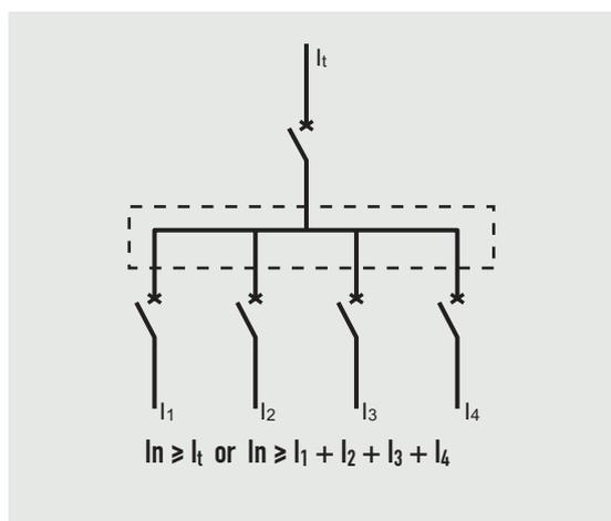
125 A modular distribution block equipped with an additional neutral terminal block >
