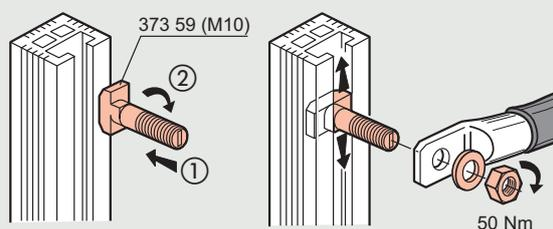
The lugs or flexible bars connect directly with no need to add washers or spacers
