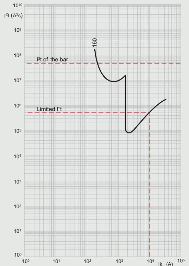
**Example:** using a 12 x 4 mm rigid flat bar for 160 A
