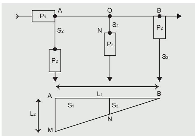
$S_1$  corresponds to the cross-section of the main conductor and  $S_2$  to the cross-section of the branch conductor.
