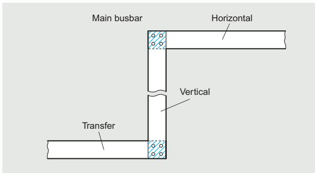
For branch busbars, the contact area can be smaller, complying with the condition  $S_c > 5 \times S_b$ . For equipment connection plates, contact must be made over the whole surface of the plate for use at nominal current.
