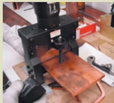
Bending a 10 mm thick copper bar on a portable hydraulic tool
