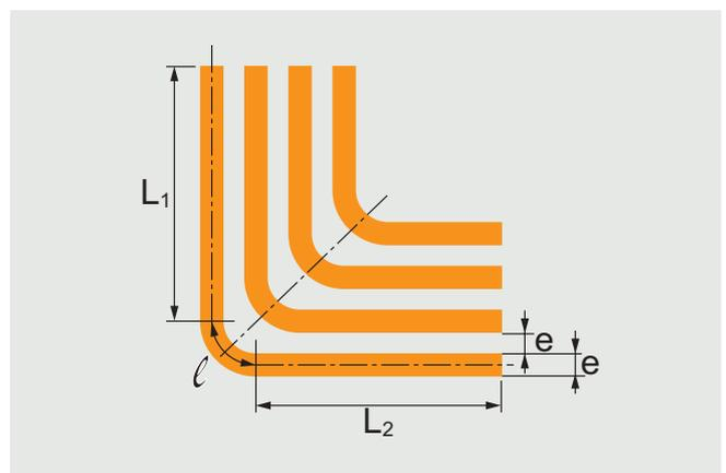
The bars are separated by their thickness "e". The total centre line length before bending is the sum of the straight parts ( $L_1 + L_2$ ) that are not subject to any distortion and the length  $l$  of the curved elements on the neutral line (in theory at the centre of the thickness of the metal).
