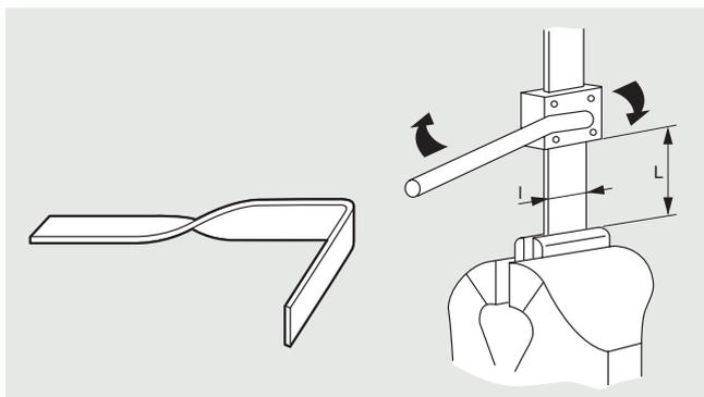
^ Creating a twist. The length  $L$  of the twist is at least twice the width  $l$  of the bar
