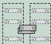
Equipotential link between two boxes using strips provided
