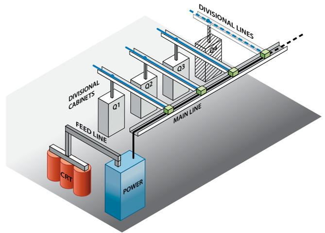
^ "Cable" solution: addition of a new distribution board to a junction box provided for this purpose
