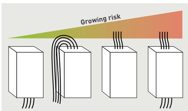
Layout of cable entries, from most suitable to least suitable
