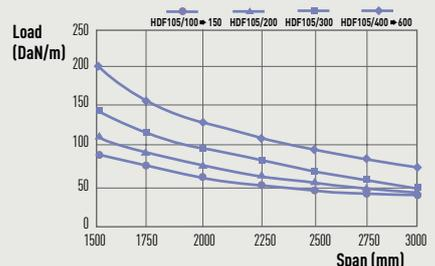
Permissible load for a deflection no greater than 1/200 with the coupling at 1/5 of the span
