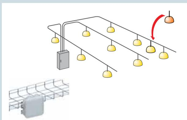
^ Lighting powered by cables in cable trays
