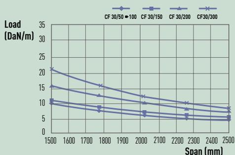
Example: diagram for 30 mm high Cablofil cable tray
