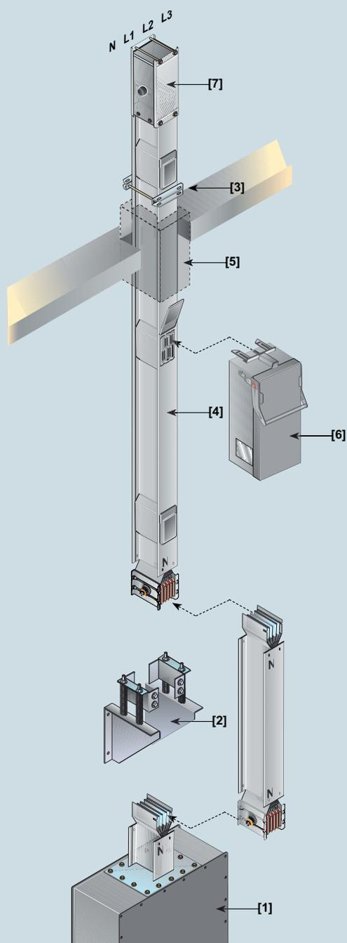
High and medium power trunking can be used in a rising main to provide vertical energy distribution in buildings.
