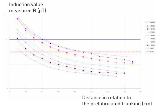
The studies conducted on the whole range show a very low level of emissions, meeting the strictest specifications, even at reduced distances: value for  $10\mu\text{T}$  (blue line) and target value of  $3\mu\text{T}$  (red line).
