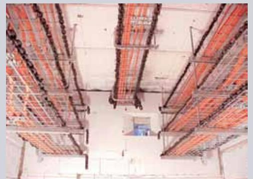
Cablofil cable trays inside the oven before the test
