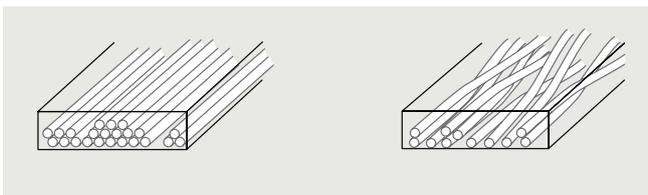
Dense, tight and compact layers are the least likely to catch fire, but in turn their capacity for heat dissipation is lower, which can lead to reduced current-carrying capacity.
