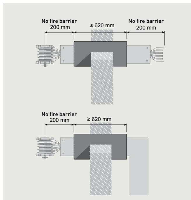
Fire barriers are a minimum of 620mm in length and must always be centred in the fire partition or flooring which is fed through. Once the fire partition or flooring is fed through, the openings must be carefully filled with material which complies with the appropriate fire safety regulations for the building.
