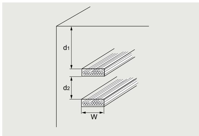
It is advisable to position layers beneath ceilings at a distance  $d_1 > 2 \times W$  (at least twice the width of the cable tray). In the event of fire, this will in part prevent a situation where the cables are positioned in the hottest of the gas layers. In order to prevent fire spreading from one layer to another, a minimum distance of  $d_2 > W$  is also advisable.
