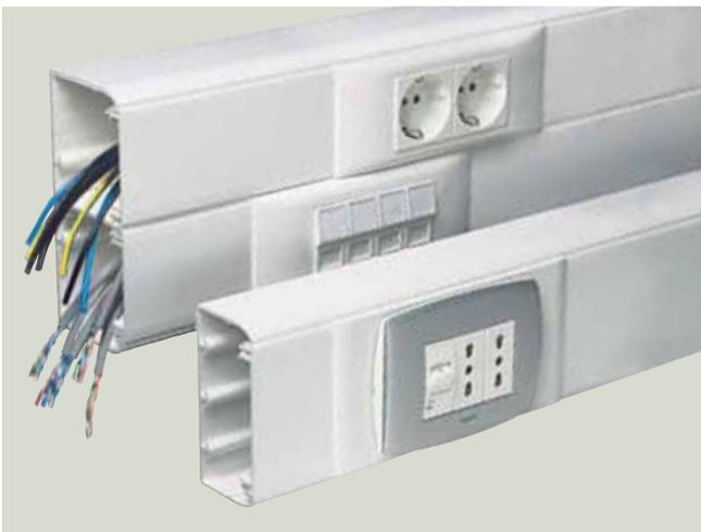
Its appearance and performance features vary according to its intended use. Although there are models made of metal, the vast majority of terminal distribution trunking units, presented in the form of skirting trunking, columns or mini trunking, are made of extruded PVC. The protection class is limited to IP 40 or 41 and impact resistance to IK 07.
