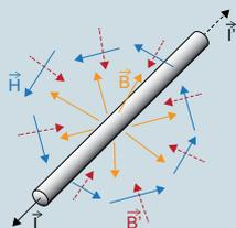
In the diagram opposite, the induction  $\vec{B}'$  generated by the field  $\vec{H}$  induces a self-induction current  $I$  which is opposed to the current  $I$  which originated it. Nothing prevents the self-induction (or own mutual induction) effect.  $L$  is approximately  $1\mu\text{H/m}$ .
