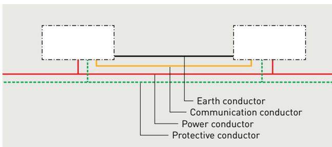
Too close cohabitation of conductors leads to couplings and the transmission of interference. Conversely, their being too far apart leads to poor equipotential and the creation of high surface loops.
