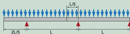
Test configuration: coupling at  $1/5^{\text{th}}$  of the span L
