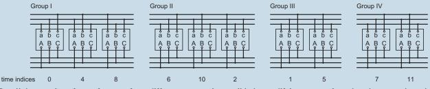
Parallel operation of transformers from different groups is possible by modifying connections, but they must be submitted for the approval of the manufacturer.
