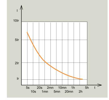
Overload capacity of an oil transformer
