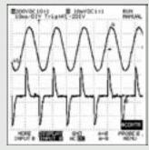
The current is ahead of the voltage and the load is distorted. Here too, the  $\cos \phi$  has no significance. The power factor is less than 1 and must take account of the reactive power (due to the phase shift) and the distorting power.
