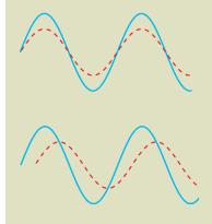
Example 1: Current and voltage in phase and sinusoidal  $PF = \cos \varphi$  and PF = 1
