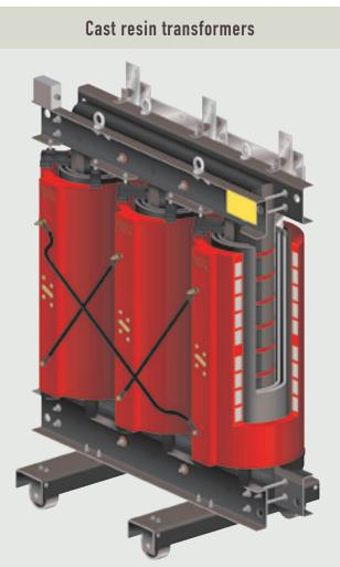
The magnetic circuit is insulated (or coated) in insulating resin. Cooling takes place in the ambient air with no intermediate liquid. of their reliability, their lower environmental impact compared to oil transformers, and because they reduce the risks of fire and spreading polluting substances in the environment.
