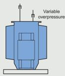
The tank is completely filled with liquid dielectric and hermetically sealed. There is no risk of oxidation of the oil.
