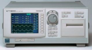
Measurements of powers (P, Q, S, D) and other data or electrical values (U, I,  $\varphi$ ,  $\lambda$ , etc.) can be easily distorted with complex signals. Numerous characteristics: permissible peak factor for an rms measurement, frequency pass band, sampling period, synchronisation (internal clock), update between two displays, must be known and controlled before taking measurements, which are quickly likely to be risky. Only suitable wattmeters or power analysers can provide this control.
