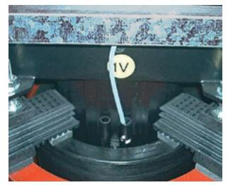
**^** PCT sensor to check the temperature
