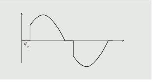
In the expression  $S = \sqrt{P^2 + Q^2 + D^2}$  the distorting power D is not zero and can be calculated, in the same way as P and Q, as a function of the non-conduction angle  $\Psi$ : the rms voltage and current, in the load, are expressed as a function of the same angle.
