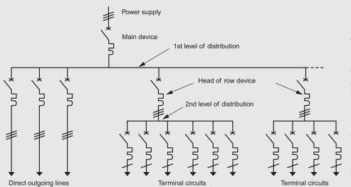
In most secondary or terminal distribution panels (see generic diagram on page 3), it is necessary to distribute three-phase and single-phase circuits. Some can supply receivers directly (direct outgoing lines) or supply points of use or small modular consumer units. In this case, it is not possible to keep to a single rule to determine the coincidence factors.
