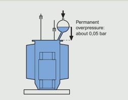
To limit the previous disadvantages, an expansion tank limits the air/oil contact and absorbs the overpressure. However the dielectric continues to oxidise and take in water. The addition of a desiccant breather limits this phenomenon but requires regular maintenance.
