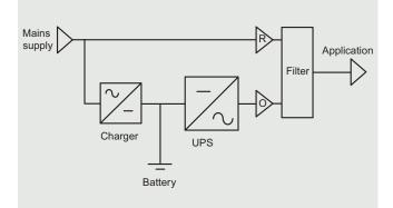
This technology is used for low powers that do not exceed a few kVA. The load (application) is supplied directly by the network via a simple filter that attenuates the disturbance.
