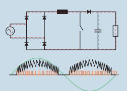
PFC is a mechanism that uses appropriate switching (shown in orange) to consume an almost sinusoidal current that is in phase. At 50 Hz, the load is equivalent to a resistor. The voltage on the capacitor is set to a value greater than the mains supply peak (typically 400 to 450 VDC).
