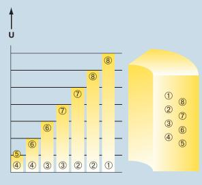
Winding made with wire conductors: the voltage increases with the number of turns
