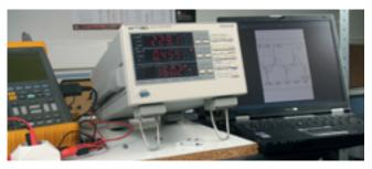
This device is used for measuring power. Current digital models can be used to access all values: P, Q, S, U; I,  $\cos \varphi$ , PF (power factor), etc., and even harmonic and frequency values. Some even carry out direct energy calculations by integrating the measurement time. These are referred to as power analysers.
