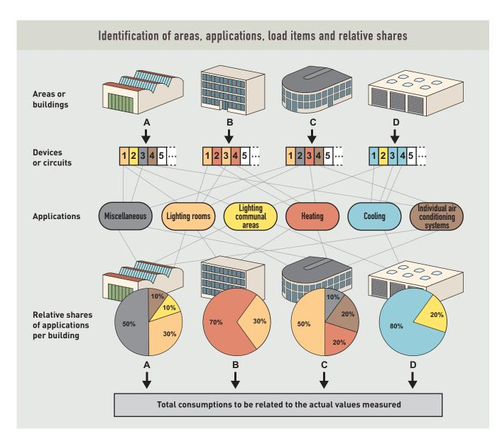
windows, offices, corridors, shelves, storerooms, cloakrooms, etc. It can be seen immediately that the measurement of all the consumptions by all the applications will reveal the challenge. Choices, sometimes arbitrary, must be made to select only high consumption applications or those which would a priori be wasteful.
