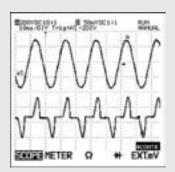
The voltage and the current are in phase but the current is not sinusoidal. The  $\cos \phi$  has no significance. The actual power factor is less than 1. Distorting power is consumed.
