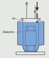
A quantity of air enters the surface of the oil and the cover allows the liquid to expand with no risk of overflowing. The transformer "breathes", but the humidity of the air mixes with the oil and the dielectric strength deteriorates.
