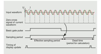
Timing of measurement based on digital sampling method
