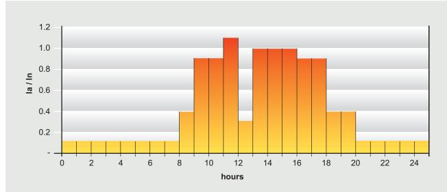
Load diagram over the working days of a small industrial factory | Ia: current effectively absorbed by the transformer In: transformer rated current | G (working days): 220
