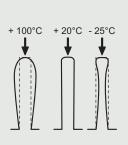
The overpressure due to the expansion of the liquid is absorbed by the folds of the tank.
