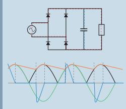
The principle is to rectify the mains supply, filter it and then install a switching device downstream that behaves like a resistive load.
