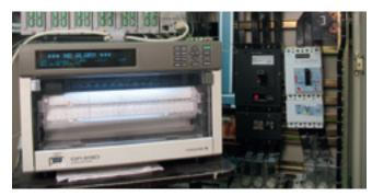
Small standalone thermometers are available that carry out repetitive measurements (for example, every two minutes) and calculate the average per period. The values are stored in the memory. More sophisticated devices such as measurement control units can acquire a wide variety of data, including the temperature, over hundreds of points. Their installation and connection are more complicated, but some can now be interfaced on a local area network or even the Internet.
