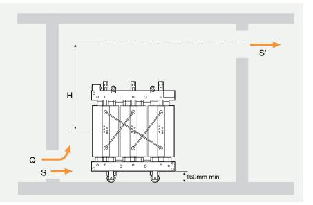
If the transformer room is small, or badly ventilated, use forced ventilation. This is also necessary when the average annual temperature is higher than 20°C or when there are frequent transformer overloads. To avoid affecting the natural convection in the room an air extractor may be installed in the upper opening, possibly controlled by a thermostat.
