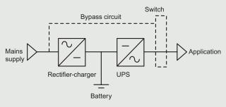
The "bypass" circuit enables the mains energy to be used
