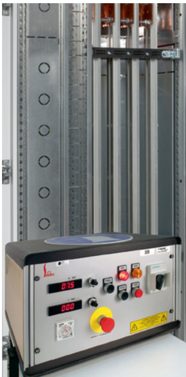
Industrial frequency > generator for insulation test
