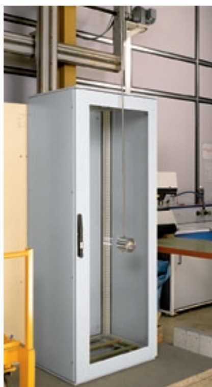
< Pendulum impact test on an Altis enclosure
